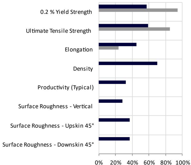
Bar plot is generated by normalizing typical material data (containing both horizontal and vertical data) against a range defined for each material family. For high strength aluminum-based alloys, the ranges are as follows: 0.2%YS: 0-500 MPa UTS: 0-600 MPa, Elongation: 0-50%, Density: 99-100%, Productivity: 5-60  $\text{cm}^3/\text{h}$ , Surface Quality (all): 5-40  $\mu\text{m}$ . 0% in the bar plot indicates the lower range value, 100% indicates the upper range value
